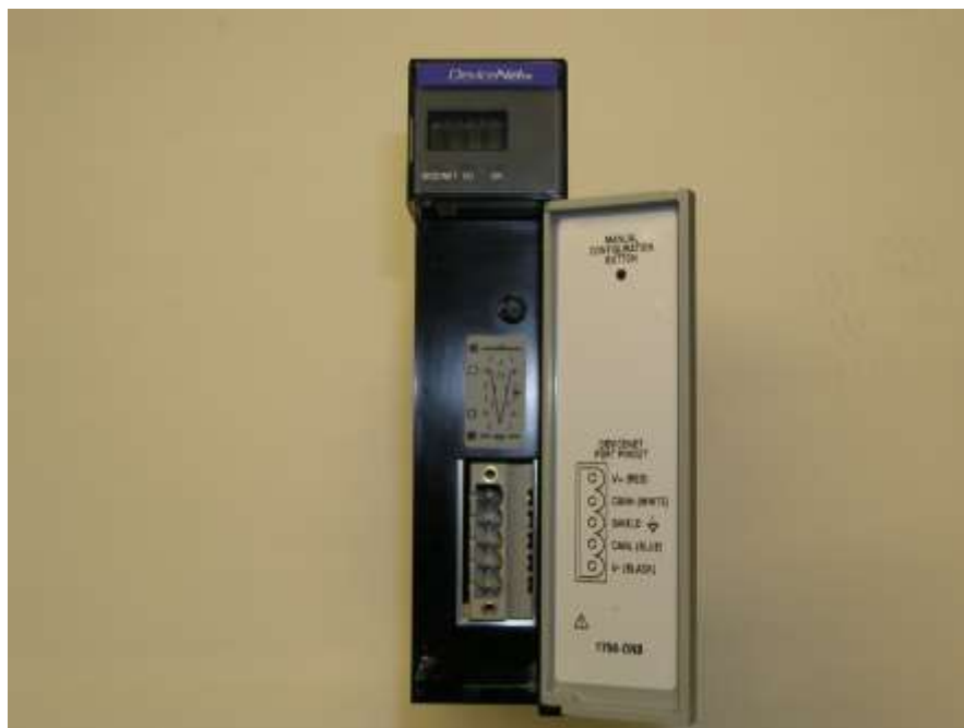
Figure 1-A ControlLogix 1756-DNB Scanner Module
