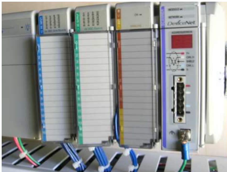
Figure 3-A CompactLogix 1769-SDN Scanner Module
