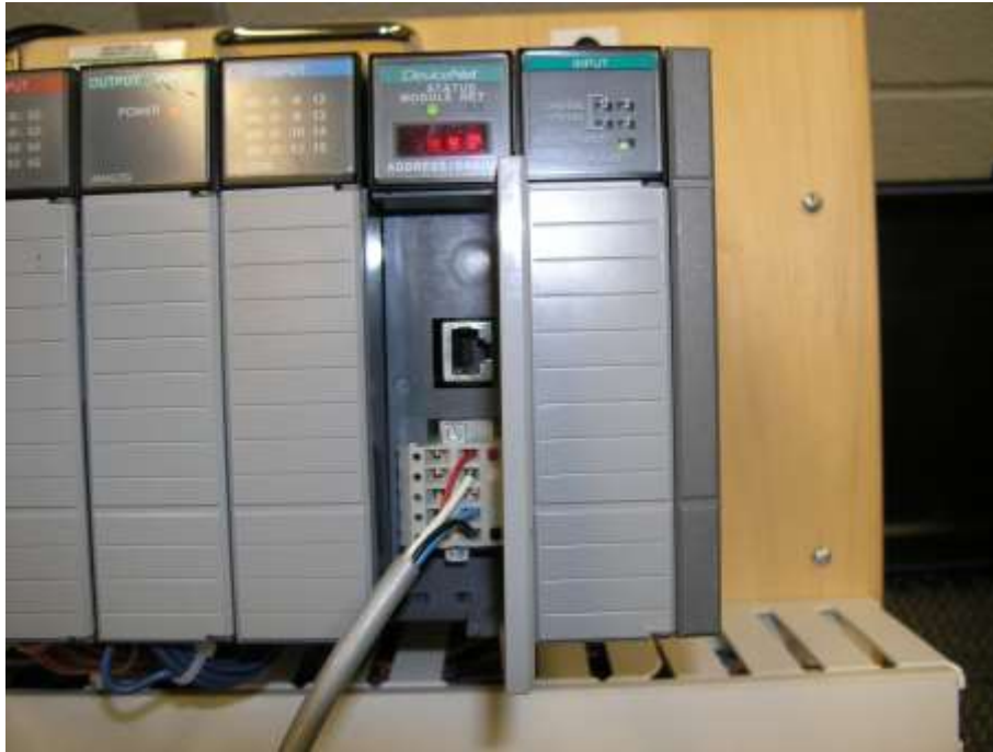
Figure 2-A SLC 500 1747-SDN Scanner Module
